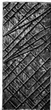
FIG. 175. Arrangement of fractures in glass plate broken by torsion. (Daubrée.)
